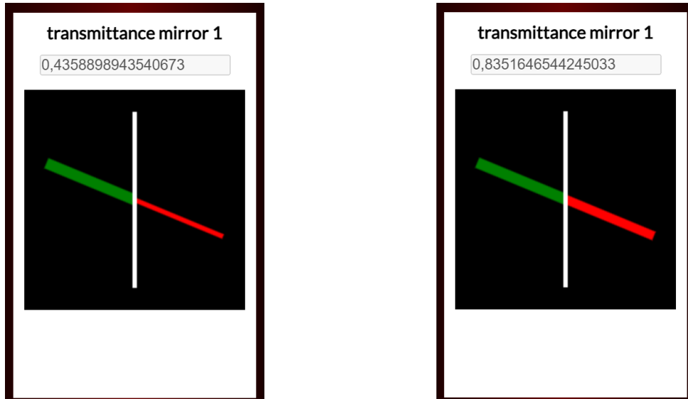
Figure 39: transmittance component , an output component that calculates the transmittance from the reflectivity of the corresponding mirror, the angle of the rays in the visualization is for demonstrational purposes only
