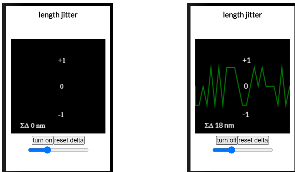
Figure 38: length jitter component , a component that randomly adjusts the movable mirror when active (right) to simulate noise, keeps track of the total delta of the position
